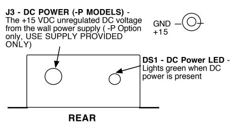
Figure 2.3 2006-11, -12 Input, Output, Power LED, External DC In (-P Option)
